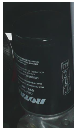
Figure 13.4.6 Compressor oil filter part number 099-008-S
