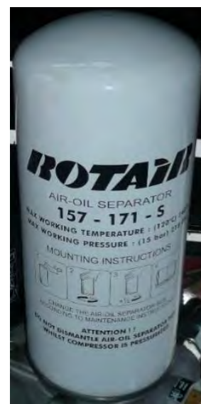
Figure 13.4.7 Oil mist separator filter
