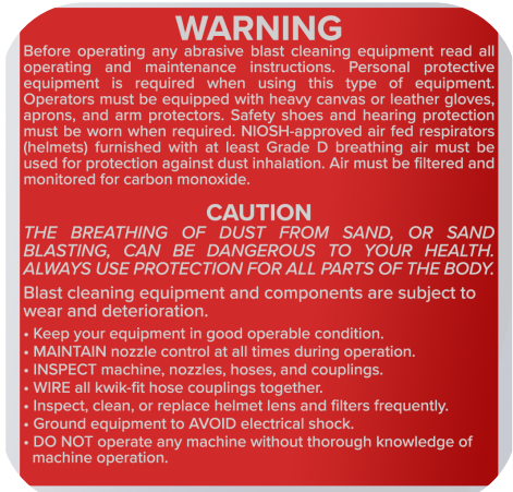
Figure 1.1 Blast pot warning label
