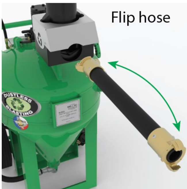
Figure 9. Flipping the pinch hose
