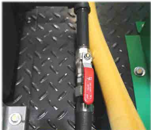
Figure 6. Valve is pictured in the open position
