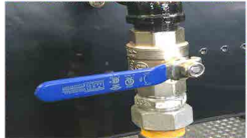
Figure 7. Valve is pictured in the closed position
