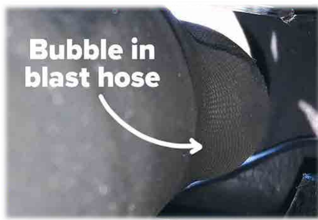
Figure 8. Bubbling in a blast hose
