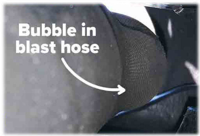
Figure 8. Bubbling in a blast hose
