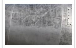
At least 2/3 of the surface should be bare metal, free of visible residue. Only tightly adhering coatings remain.
