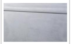
Free of all visible paint, rust, mill scale, stains, and foreign matter. Steel will actually be grey, not white.
