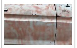
Only tightly adhering residues can stay. All loose rust, mill scale, and coatings must be removed.
