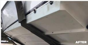
"Two layers of bottom paint melted off with the Dustless Blasting machine. Left the perfect profile for a new layer of bottom paint **that will last.**"
