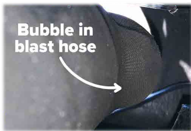
Figure 8. Bubbling in a blast hose
