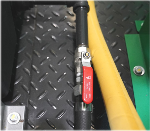
Figure 6. Valve is pictured in the open position
