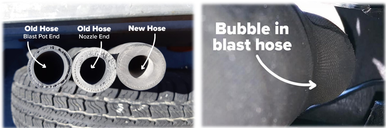
Figure 8. Bubbling in a blast hose
