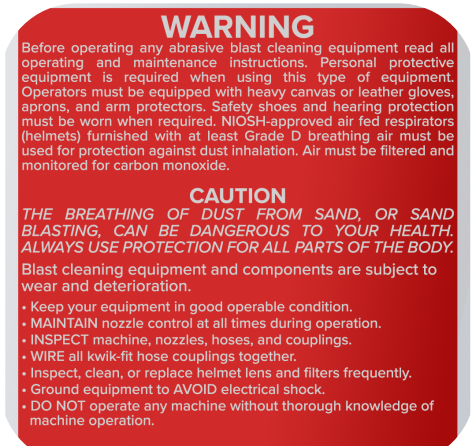
Figure 1.1 Blast pot warning label
